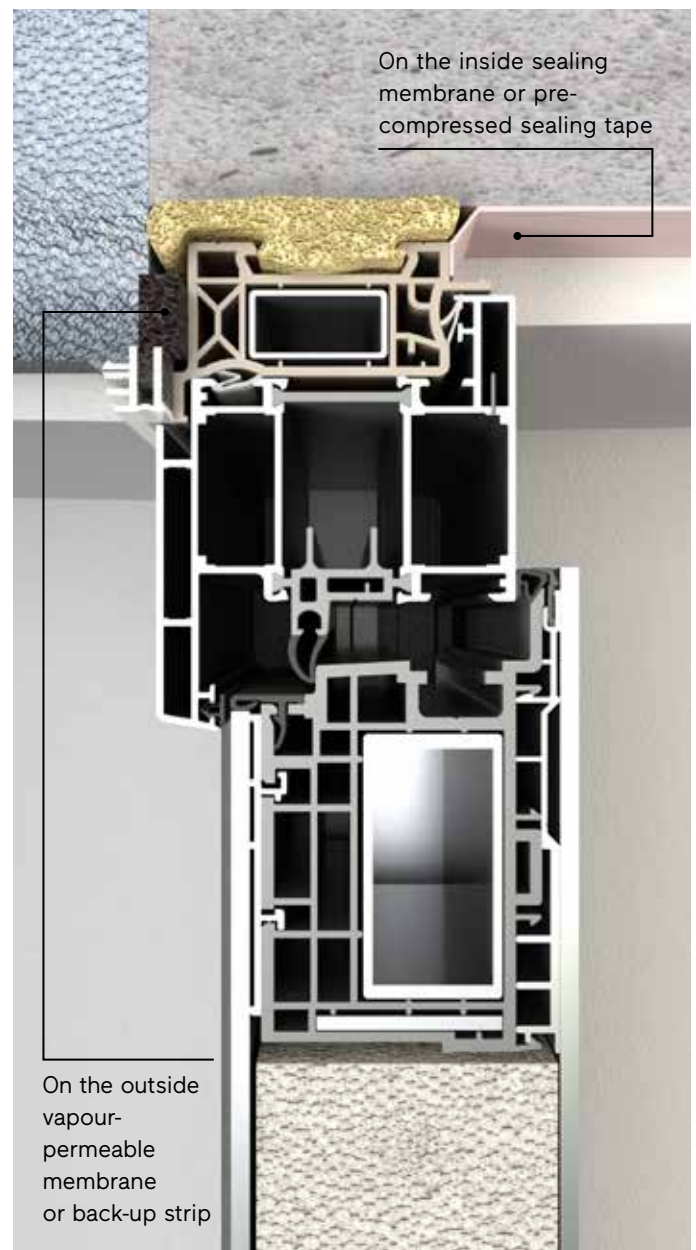
Two-stage installation with frame
