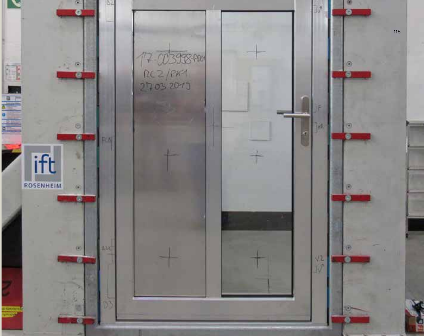
The burglar resistance of doors is investigated at a test stand at the Institut für Fenstertechnik (ift) Rosenheim.
